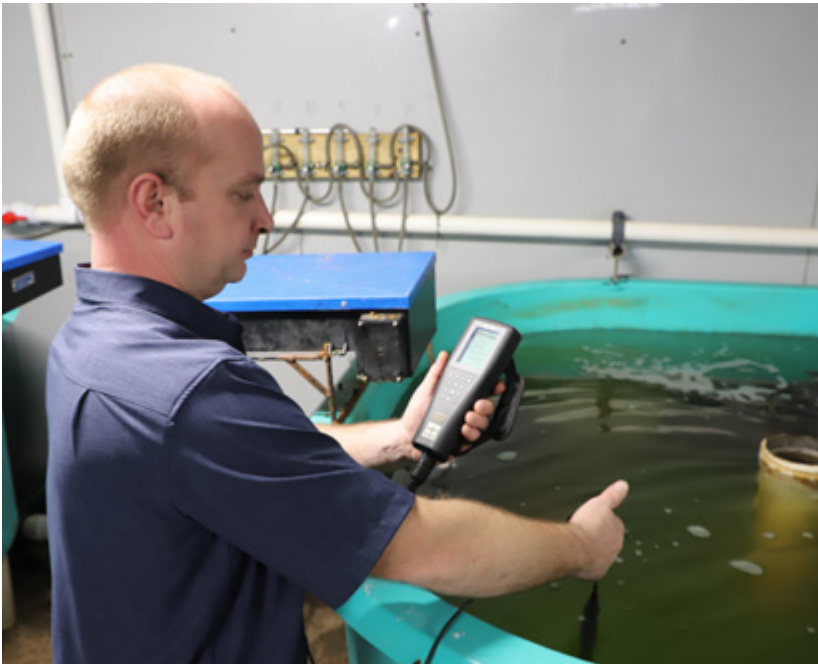
Leland uses the ProODO handheld to spot check DO and temperature in one of the facility tanks
